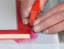
3: Using a sharp knife or scalpel, cut the mesh away from the outside of the frame then release the mesh edges from the rack screen stretcher. The screen is ready to mask.
