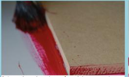
2: Lay a board or piece of card the same size as the inner area of your frame on top of the mesh. Using a stiff, short bristled brush, paint mesh adhesive onto the frame by applying onto the areas where the mesh is in contact with the frame. Hold the board/card on top of the mesh in place whilst painting the adhesive on to protect the screen printing area of the mesh, then remove it whilst the adhesive is still wet. Leave the adhesive to dry thoroughly.
